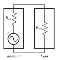
Figure 8.3. Effective circuit for a receiving antenna.
