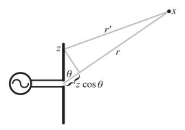
Figure 8.1. Center-fed dipole antenna.
