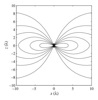
Figure 8.2. Radiation from a half-wave dipole.
